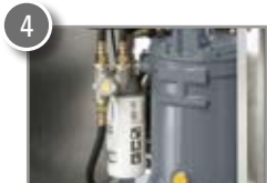
Oil separator & oil filter
