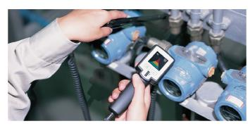
5. To find the exact location of the leak screw the focus tube and the focus tip on the sensor.
