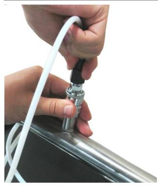
2. Connect the other end of the teflon hose with a quick connector. The teflon hose with quick connector is used to connect the S 130 to the process.
