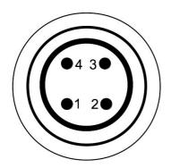
Connection pins (view from the clamping side)
